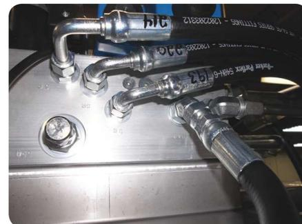
The upgrade includes stainless steel hose ends and fittings on all hydraulic hoses and high-pressure water lines for the following models: SSFIT-EV1, SSFIT-425, SSFIT-425-5HP and SSFIT-425-10HP.
