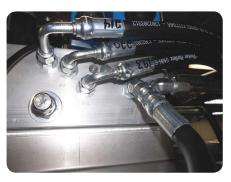
The upgrade includes stainless steel hose ends and fittings on all hydraulic hoses and high-pressure water lines for the following models: SSFIT-EV1, SSFIT-425, SSFIT-425-5HP and SSFIT-425-10HP.
