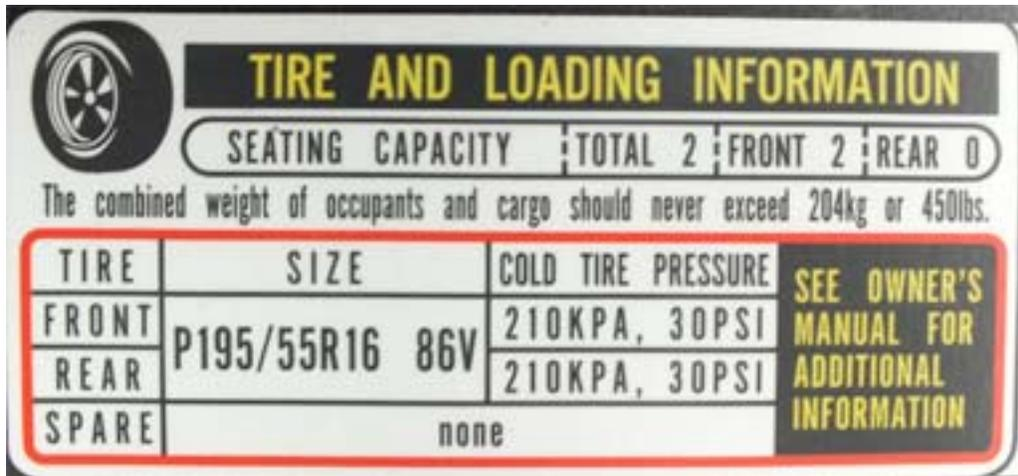
Curb weight of the Honda will be  $GVRW - \text{Tire and Loading capacity} = 3,263 - 450 = 2,813$  lbs
