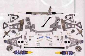
front antiroll bar with billet arms enables fine chassis tuning. Wheel hubs and all related hardware are included. The Street Performance kit for a '65 Mustang with a Windsor engine is PN GR350 SP-E-50 priced at \$6,664.45. The Street Performance rear suspension to match goes for \$3,104.60. The standard K-member accepts 302/351-style engines and Griggs Racing offers a GR350 K-member that swaps in Ford Modular engines and LSX powerplants as well.
