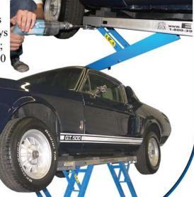
EZcarlift was developed specifically for the home mechanic. The simple operation of the common floor jack and unobstructed access of jack stands, were used as a model for the design. The true portability of the EZcarlift<sup>™</sup> distinguishes it from all other lifts.
